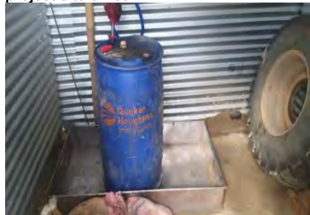
Proper storage of fuel drum. 110% containment volume metal tray noted.
